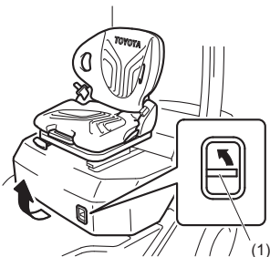
(1) Engine hood lock release lever
